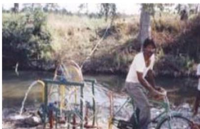
Fig-1 Bicycle operated centrifugal pumpset
