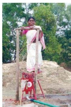
Fig-2 Pedal operated reciprocating pump
