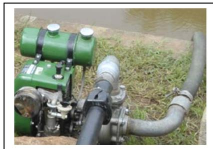
Plate-3 Portable Diesel Pumpset of 1.5 Hp
